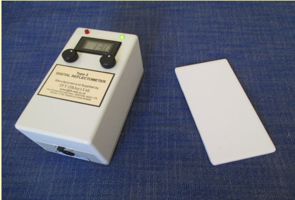
Image 2 - Reflectometer and Ceramic Calibration Tile.
