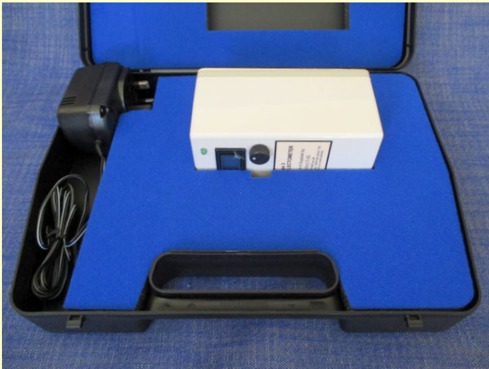
Image 1 – A Reflectometer and Fast Charger in the Protective Carry Case.
